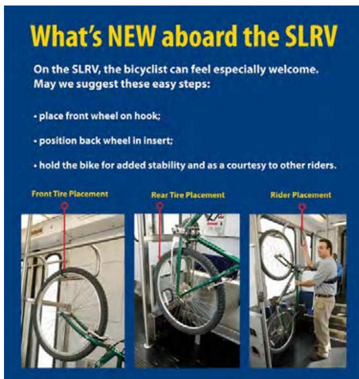
Figure 4.13: Instructions for hooking bicycle in DART's Super Light Rail Vehicle (SLRV) Image credit: dart.org
