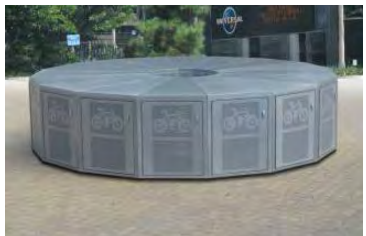
Figure 5.16: Pie-shaped bike lockers offer a more space-efficient design. Image credit: landscapeonline.com
