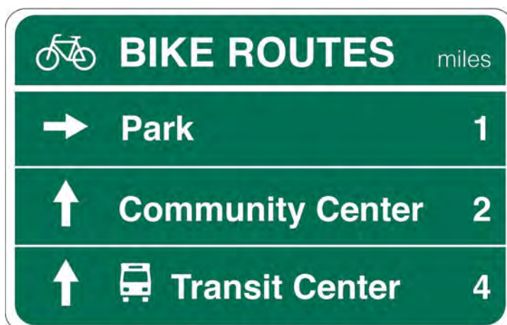
Figure 5.1: Directional signage, located prior to intersections of bike routes and paths indicate direction and distance to transit facilities, as well as other area destinations.
