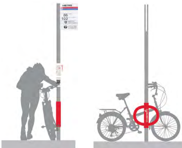
Figure 5.10: Signpost bike rack allows bikes to be locked up parallel to the curb line. Left: view as seen walking along sidewalk, right: view as seen when facing curb.
