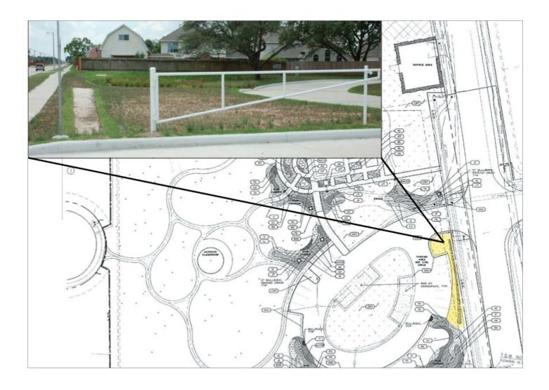
Vegetated buffer strips consist of planted or naturally occurring vegetation such as shrubs, trees, and plants. The vegetation serves as a filter, straining out sediments, nutrients, pesticides and other pollutants before they reach the stormdrain. In this case, the storm water sheet flow off the parking lot and roadway makes its way into the buffer strip where it is filtered before it enters the storm drain system. Vegetated buffer strips act as natural, living sediment and pollutants filters.
