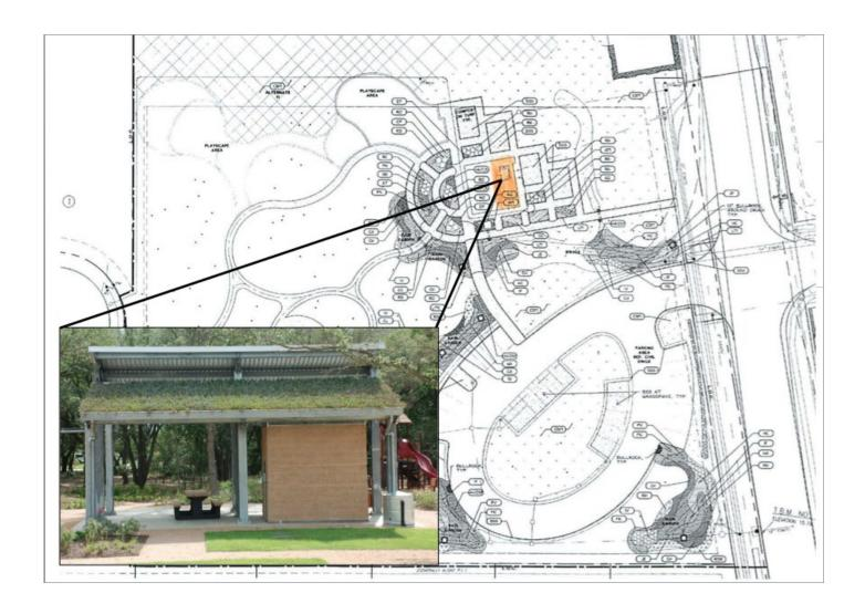
Green roofs help to manage storm water and protect water quality by reducing and slowing storm water runoff and filtering pollutants from storm water. They also act as insulators by reducing heat from sunlight and helping to lower the energy costs of cooling a building. Additionally, they provide aesthetic value to a structure while providing habitat for wildlife.
