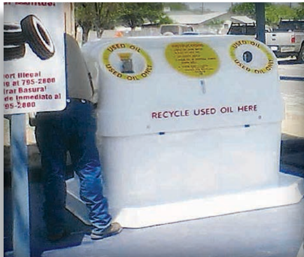
The City of Laredo purchased a 400 gallon stationary used oil collecting tank.
