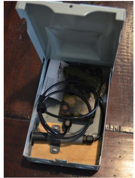
Inside of Urban Metal Box (Counter located in camouflage case, hooked up to infrared sensor)
