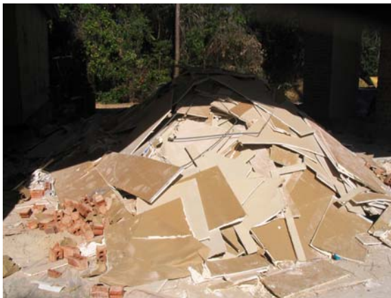
Figure 67. Stored pre-grind drywall
