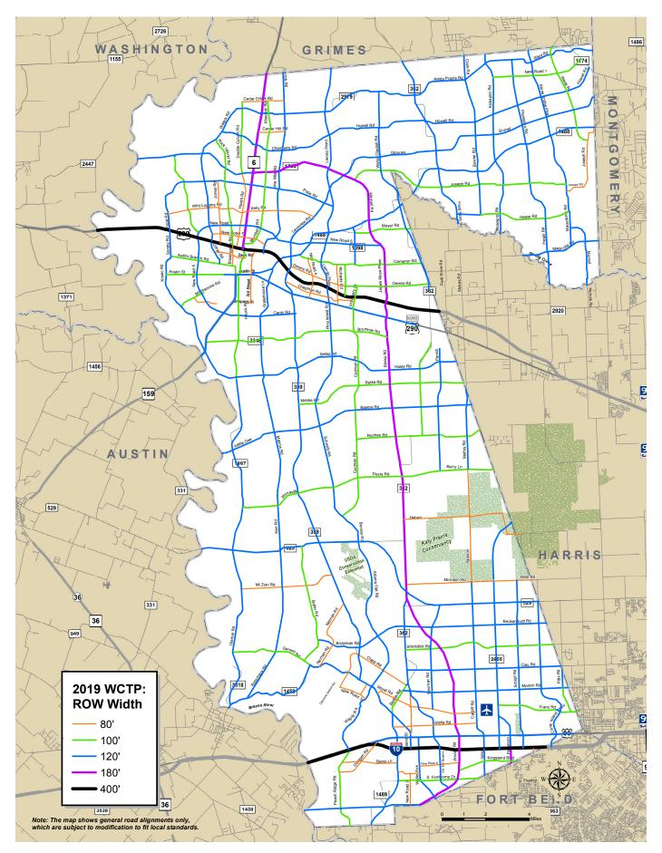
Figure 5-10: 2019 Waller County Thoroughfare Plan: Right-of-Way Widths
