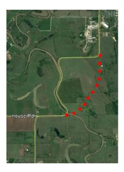
Figure 4-3: Example of Road Straightening
