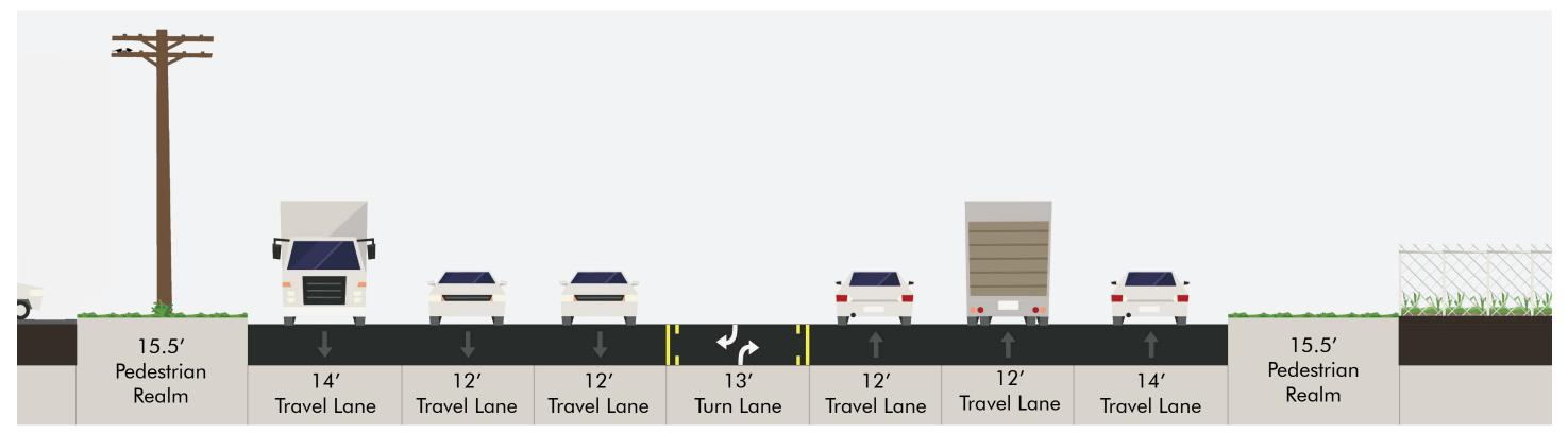
Figure 1.2 FM 1092 Study Corridor Typical Cross Section
