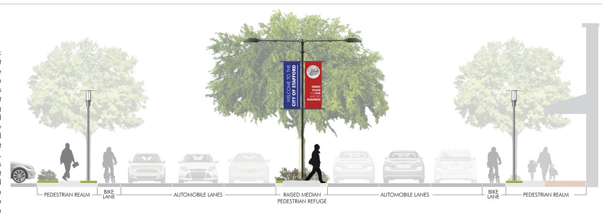
Figure 5.22: Streetscape design addresses the pedestrian realm, bicycle and automobile travel, and the right-of-way edges
