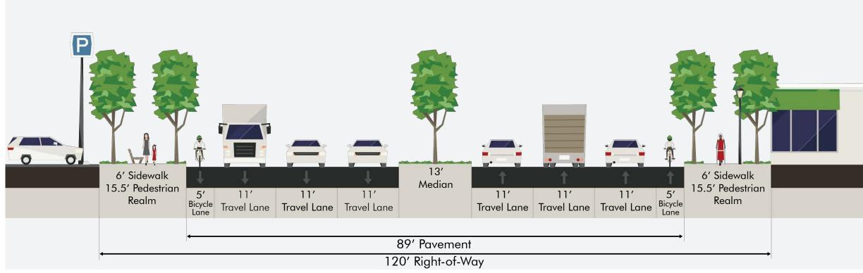
Figure ES.3 Proposed Typical Cross-section - Roark Road to Dove Country Drive
