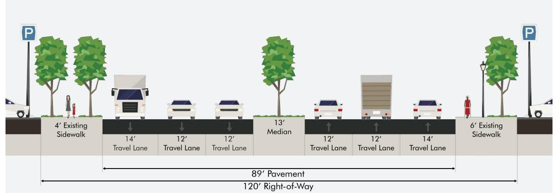
Figure 5.3 Proposed Alternative Cross-section - US 59 to Roark Road
