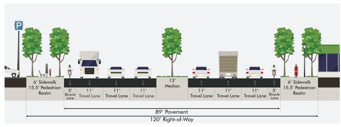
Figure 5.2 Proposed Typical Cross-section - Roark Road to Dove Country Drive
