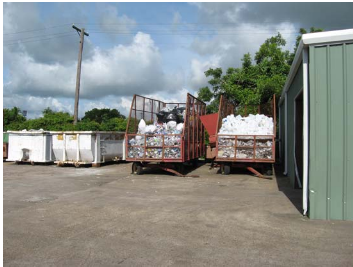
Figure 1-5: Trailers and roll-offs used for material storage
