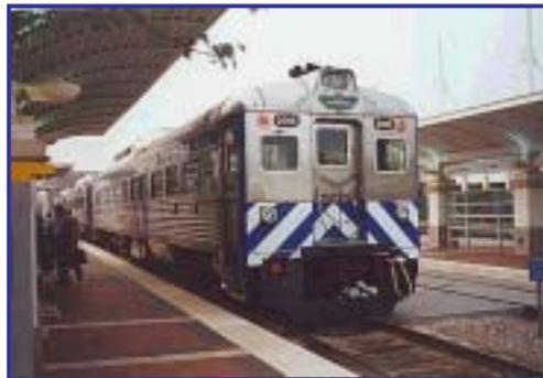
Figure 3-1 – Trinity Railway Express operates diesel locomotive-hauled coaches.
